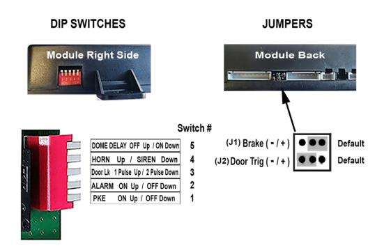
IMPORTANT: You MUST remove power from the system prior to changing any Dip Switch or Jumper settings!
