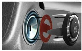
Insert cut Ignition key into lock cylinder.
