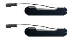
The iKey uses a sophisticated Dual Zone antenna system to allow it to effectively operate on everything from a small sub-compact to full size SUV, the systems dual antenna design guarantees consistent range and performance regardless of vehicle type. The Main Antennas generate a low frequency RF field that extends approximately 4 feet around the vehicle. When you enter this field, the low frequency RF signal triggers the iKey Fob in your pocket to transmit its authorization code to the system.
