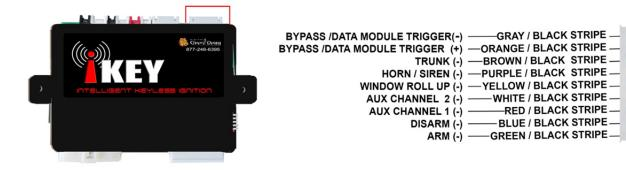
**Gray / Black wire Bypass / Data Module Trigger ( - ) 500mA** This wire is used to trigger a Transponder Bypass or Data control module with a (-) trigger. This wire provides a constant Negative output while the system is in ACC, ON and START modes. This output activates 0.5 seconds before ACC 1 and can be used to activate bypass / data modules with (-) trigger inputs.
