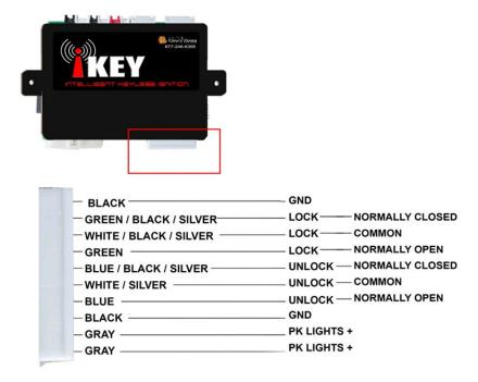
**Black wire Ground ( - )** This is the system ground. This unit requires a substantial ground to handle high current draws. **THIS WIRE MUST BE CONNECTED DIRECTLY TO THE VEHICLES BATTERY GROUND TERMINAL** or factory ground block on chassis. Note **DO NOT** use a self-tapping screw for this ground.
