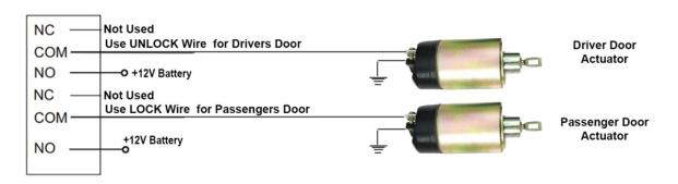
\*\*\* The iKey internal door lock / unlock relays are rated at 20A, Should your door popper actuators require a higher amperage add external relays of the correct amperage.
